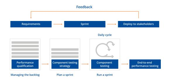
In this environment, the performance testing process should follow the workflow below.
